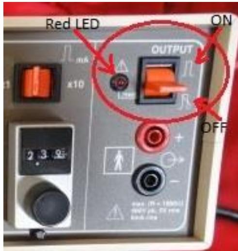
Fig 12, Output Enable Switch
